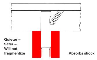
POWERTHANE'S pressures shown are as free standing when mounted wring fit pressures will be approximately 25% greater, each additional 3mm deflection increases pressure 60% up to maximum recommended deflections of 25%.
